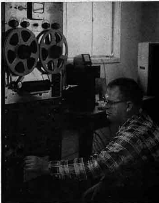
K6UAA puts the finishing touches on the tracking equipment at W6EE. Telemetry signals plus WWV was recorded on tape. A low-noise converter and ARR-15 receiver were used for tracking.
